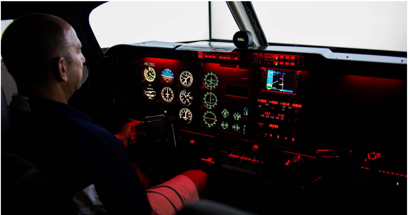
Image 3: iGATE Model G500 SEL representing a Cessna 172 with GNS 430W
