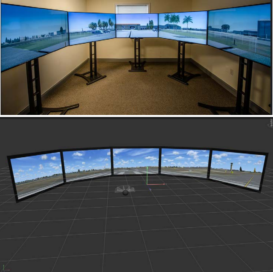
c) iGATE AATD with 5 HD TV Display Configuration (180 Degree Field of View)
