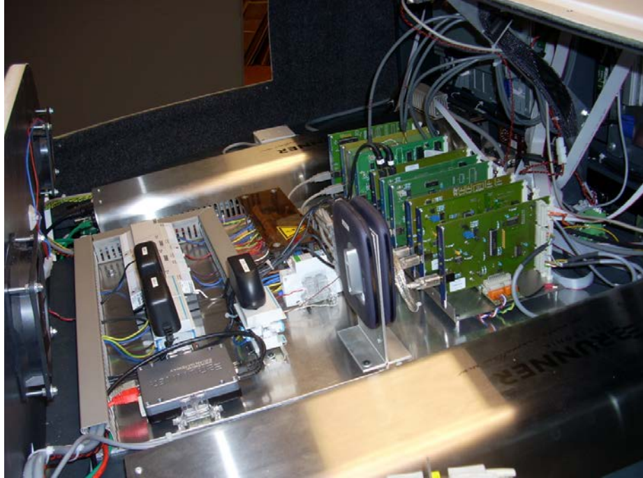
Image 14: iGATE Hardware Controllers (Masks, Switches, Flight Controls and Avionics)* *(CANBUS-style configuration and optional control loaders shown)
