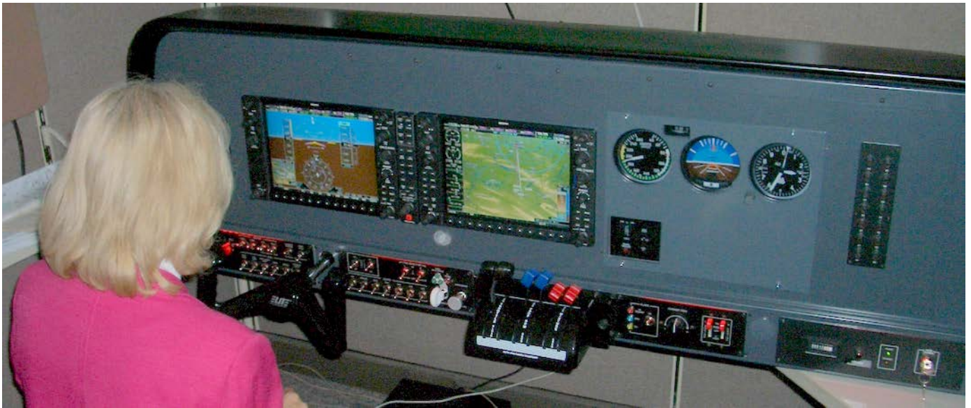
Image 10: iGATE Model G1000 SEL representing a Baron G58 Twin Open Cockpit
