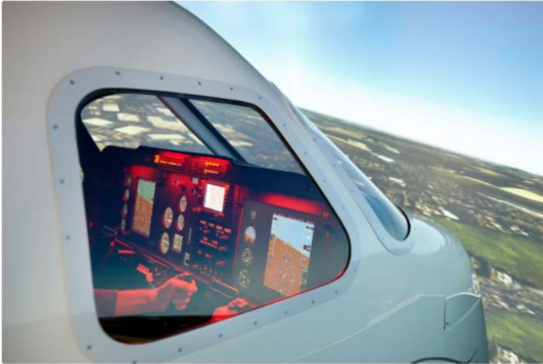
Image 2: iGATE Model G500 SEL representing a Cessna 172 with E500 AHRS and GNS 530W
