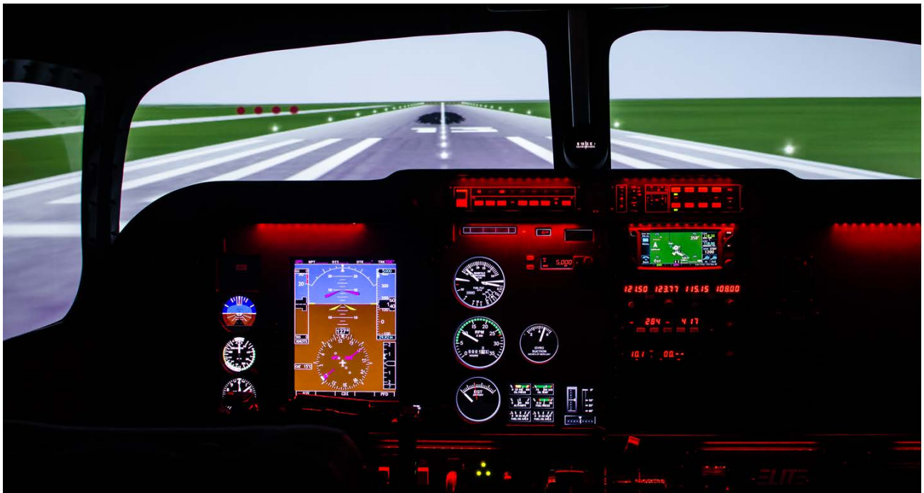
Image 7: iGATE Model G500 SEL representing a Piper Arrow with E500 AHRS
