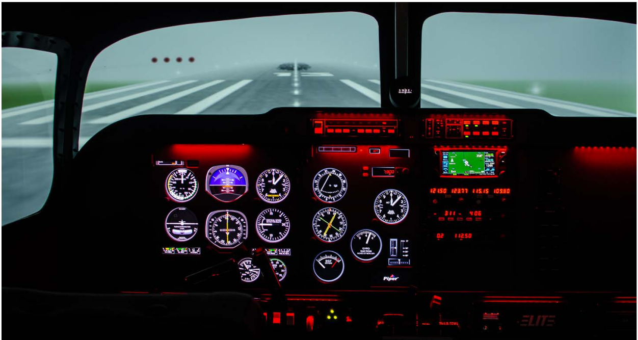
Image 6: iGATE Model G500 SEL representing a Piper Arrow with GNS 430W
