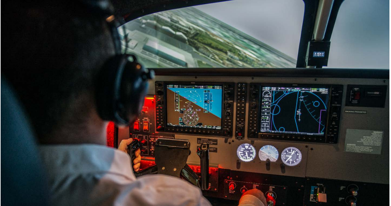
Image 4: iGATE Model G500-G1K SEL representing a Cessna 172 with G1000
