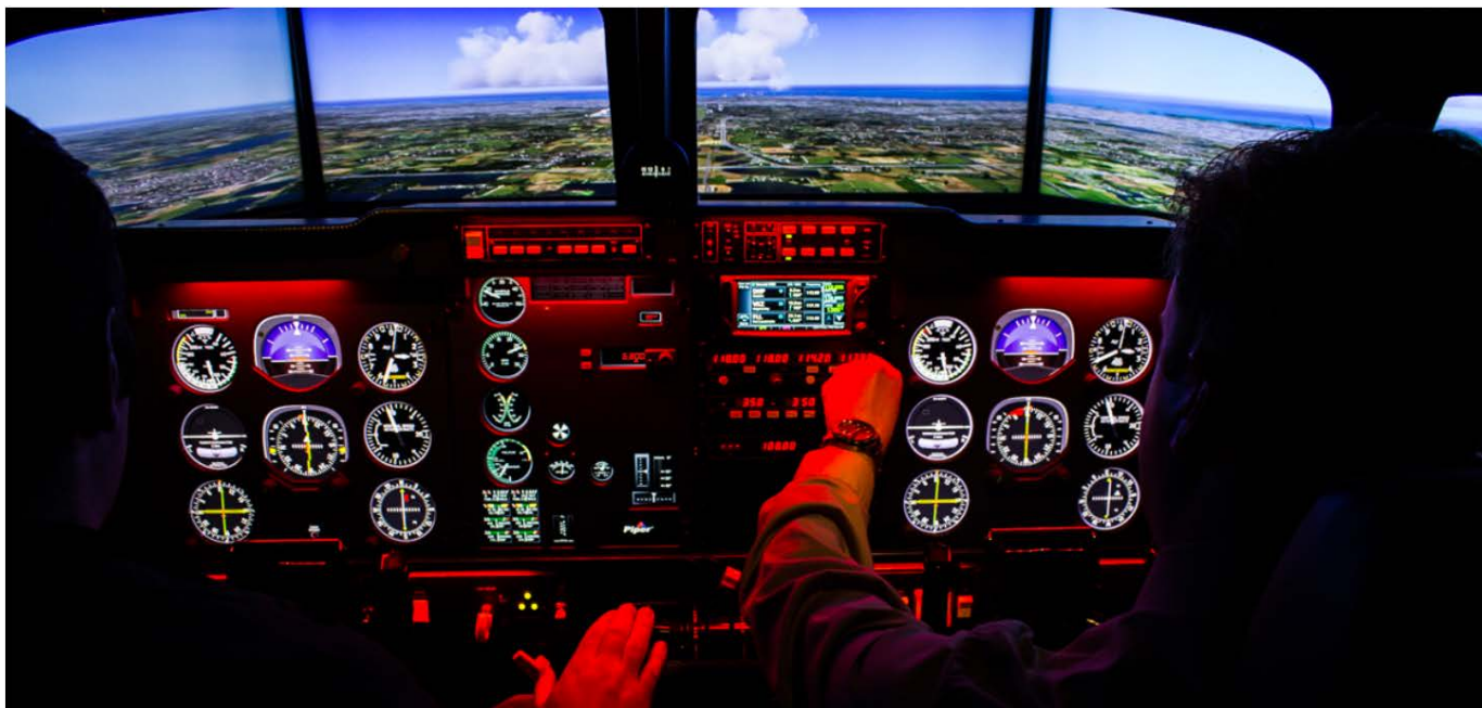
Image 8: iGATE Model G500 SEL representing a Piper Seneca Twin with GNS 430W
